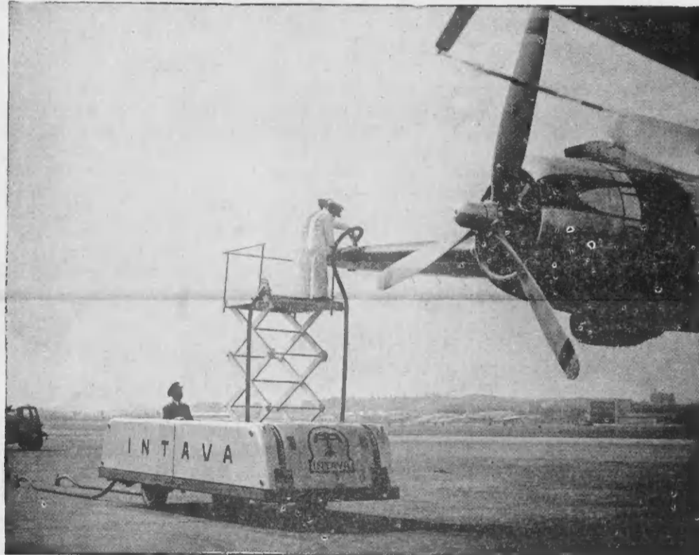
Intava, Company subsidiary for aviation business outside the United States, recently demonstrated at La Guardia Field a revolutionary new method of fueling airplanes. The Intava "Servicer" gets away from tank trucks, pumping gasoline with its own pumps direct from underground storage tanks to the airplanes. It also replaces ladders, which can damage the leading edge and de-icing equipment of a wing, with an "elevator" that lifts the refueling crew to the level of the wing.
